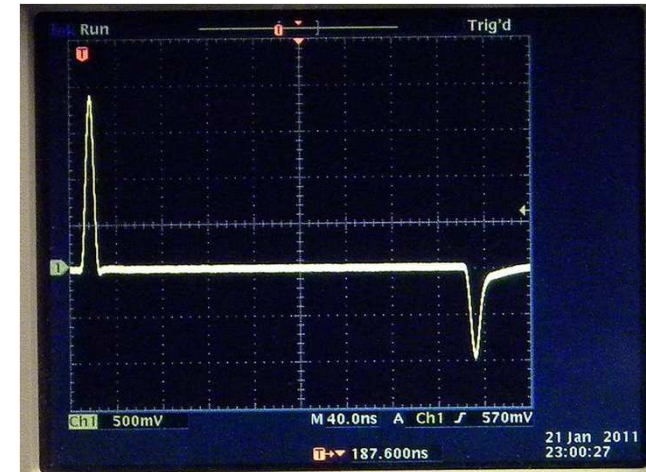
TDR: Inverted reflection
