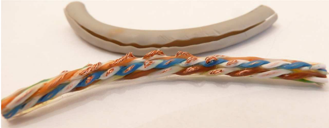
Melted cable (electrical short)
